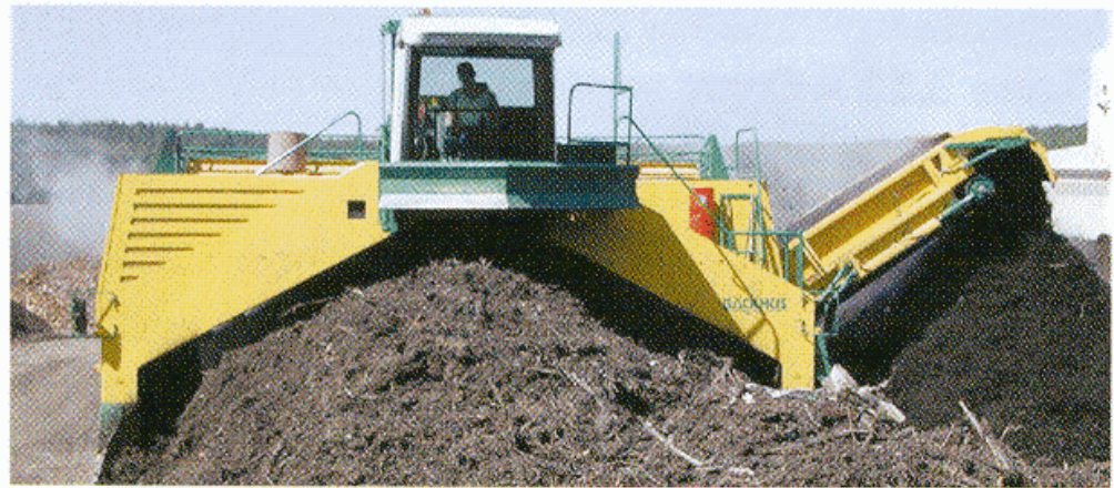
Rys. 7. Maszyna do odwracania i formowania pryzm (Bacchus) Fig. 7. Machine to turn over and formation of the compost piles (Bacchus)
