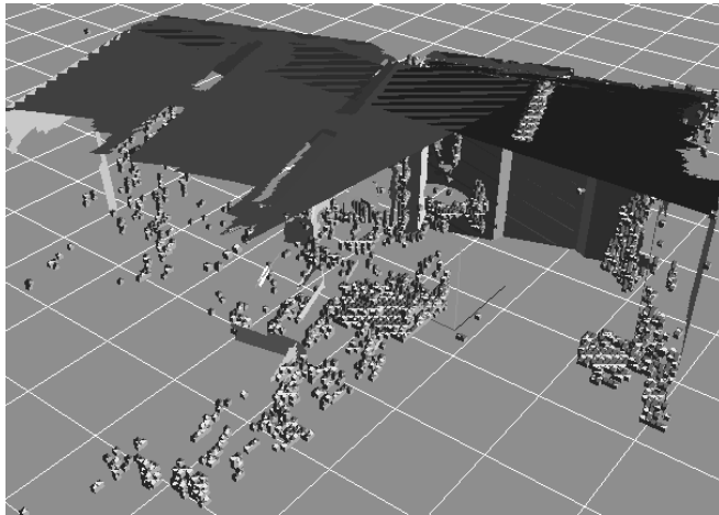
Fig. 4. The dual map: extracted planes and voxels that represent non-plane obstacles
