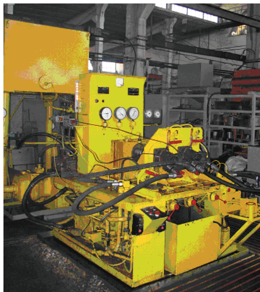
Fig. 2. The stand with recuperation of powers for tests APH 403.112
