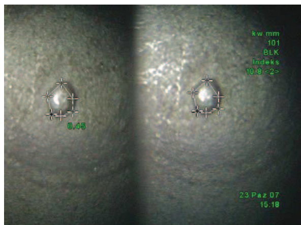
f) Surface „bulge” area measurement (closed broken line) on the blade-bed by means of „Stereo” method - 0,45 mm 2 , at measurement accuracy index 10,8, representing 0,1 mm 2
