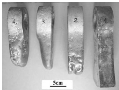
Fig. 5. A view of crusher hammers after service tests (1- at the delivery state, 2-4 after service)
