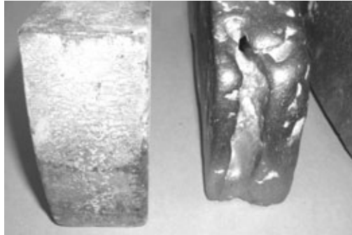
Fig. 6. A view of crusher hammers after service tests (the first hammer on the left – the delivery state, the other - after two months' in service)
