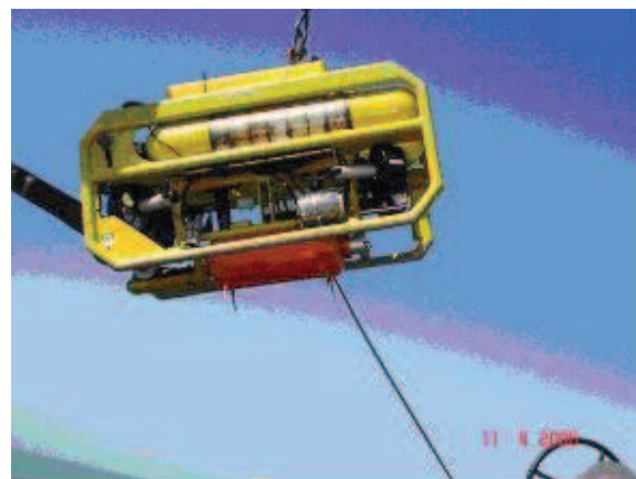
Fig. 4. ROV vehicle with TNT charge
