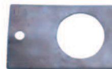
Fig. 3. The measuring orifice plane
