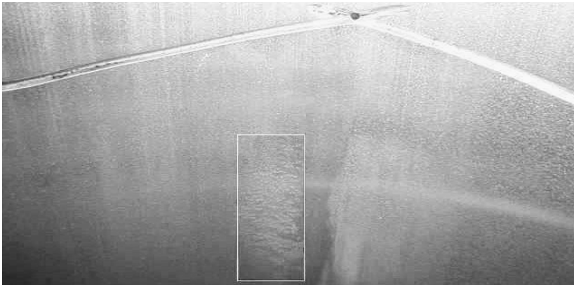
Fig. 3. Adhesive wear of cylinder liner
