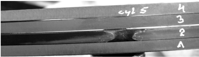
Fig. 5. Burnt part of piston ring
