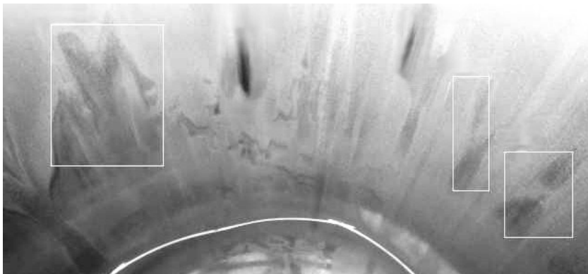
Fig. 4. Scuffing of cylinder liner
