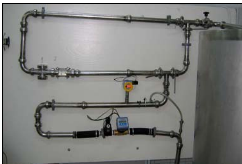
Rys. 2. Stanowisko do mycia rurociągów w systemie CIP i element kontrolny Fig. 2. Pipeline washing station in CIP system and control element
