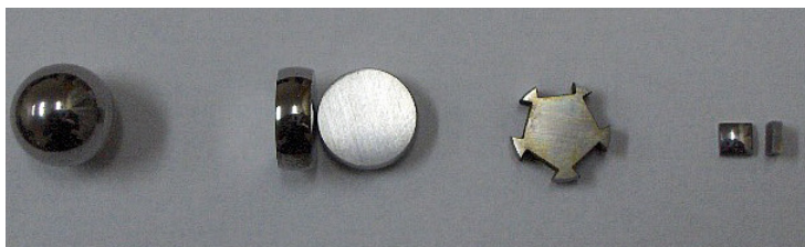
Fig. 1. Individual stages of cut samples (ŁH-15 steel)
