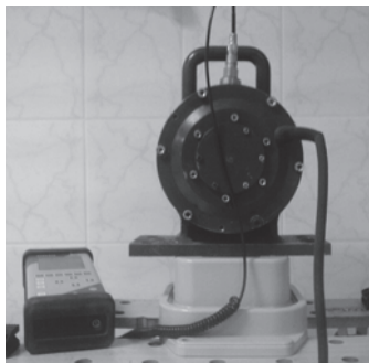
Fig. 3. Determination of the vibroisolator resonance response
