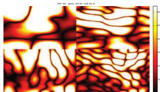
Fig. 15. Sixth level of 2D wavelet decomposition – results useless for damage detection proposed algorithm
