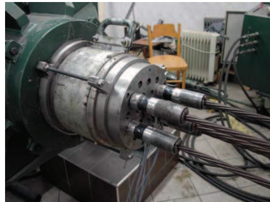
Fig. 9. View of the fasten of force sensors
