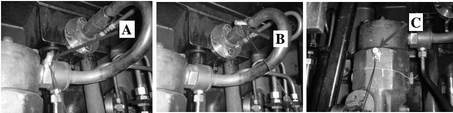
Fig. 2. Placement of the acoustic emission sensor for monitoring the signal generated by the fuel injection pump (A) and the injector (B) and the 2 nd point of the fuel injection pump (C)
