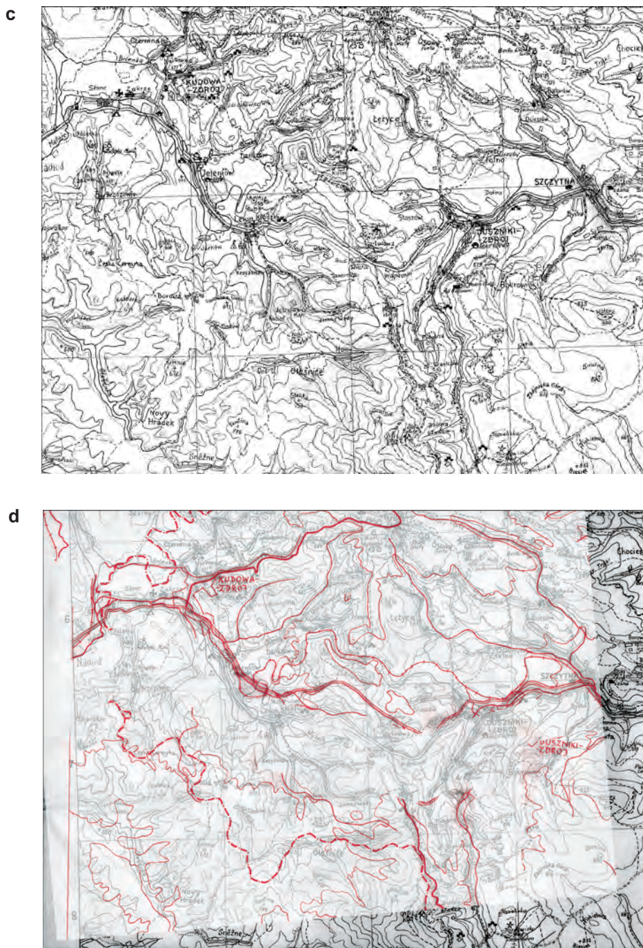
Fig. 6. Elaboration of a manuscript: a) part of a drawing of basic map elements prepared basing on source materials, prepared to be cut; b) part of assembled material prepared for censorship; c) part of a map manuscript prepared basing on the assembly, presenting an apparently faithful terrain image; d) comparison of map elements' positioning on a fragment of the assembled map (red) and the manuscript (black)
