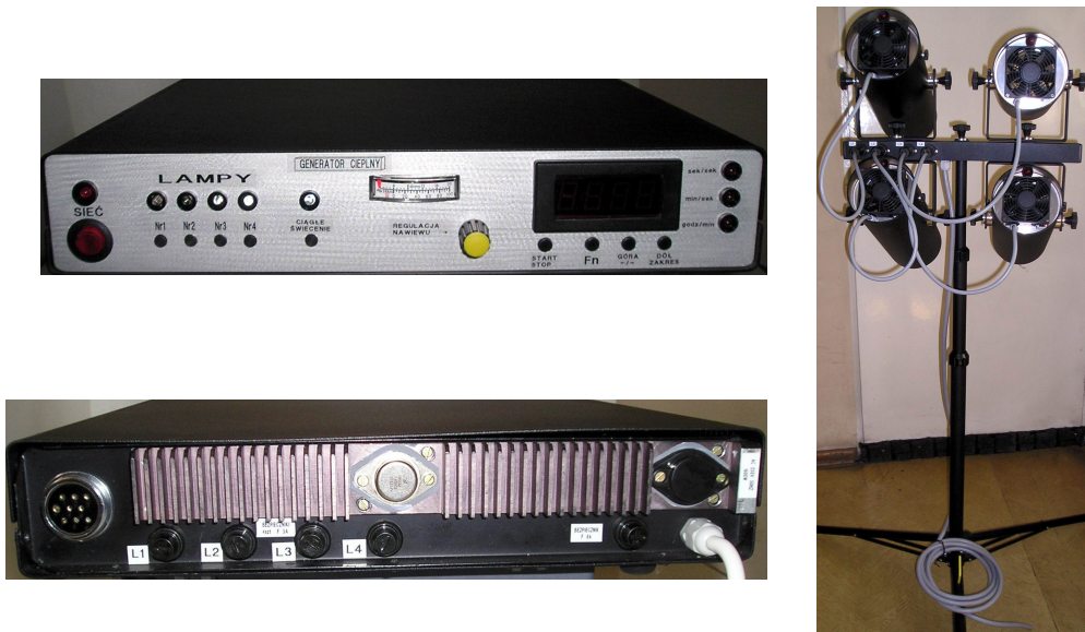
Fig. 2. Optical lock-in thermography system
