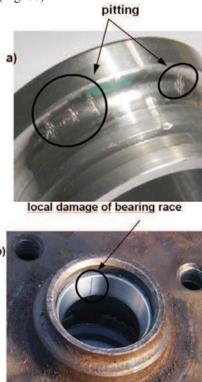
Fig. 8. Local damage of the rolling bearing race: a) operational, b) used in experimental research
