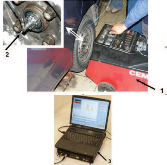
Fig. 2. Method of speeding up the wheel for the purpose of vibration measurement: 1 – on the car wheel balancer, 2 – accelerometer, 3 – measuring apparatus
