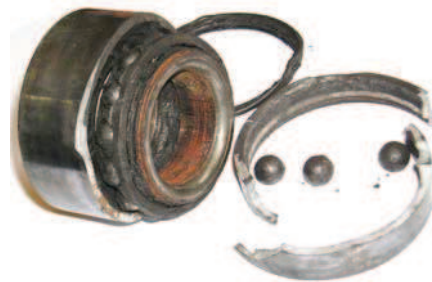
Fig. 2. Crack of the external race of double-breasted ball bearing
