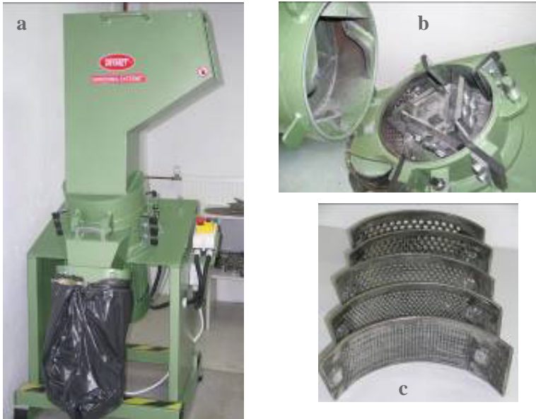
Fig. 2. T2 SW mill (TRYMET, Poland): a – overall view, b – disintegrating system, c – screens
