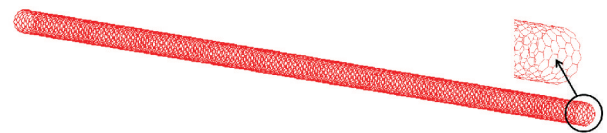
Fig. 2. FE model of a single-walled zigzag CNT
