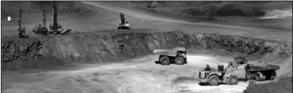
Fig. 1. A mining operation of an iron ore mine, including drilling, explosion, loading and hauling
