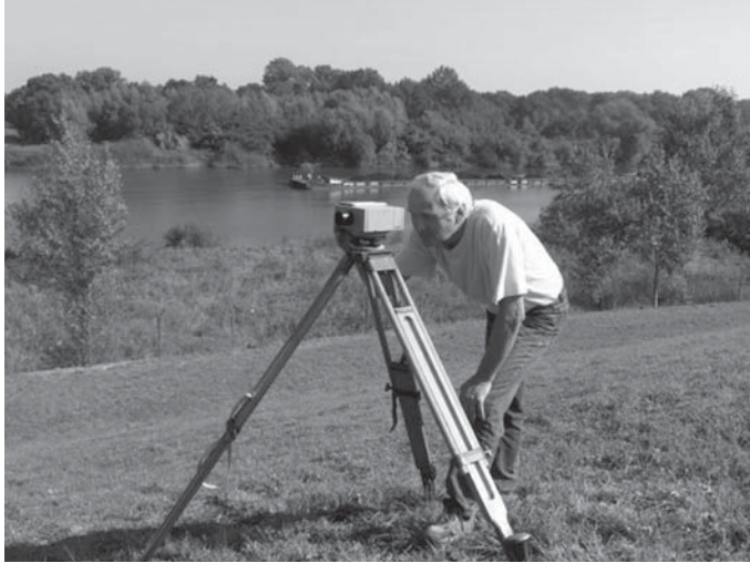
Fig. 4. The precise digital level NA 3003 during use
