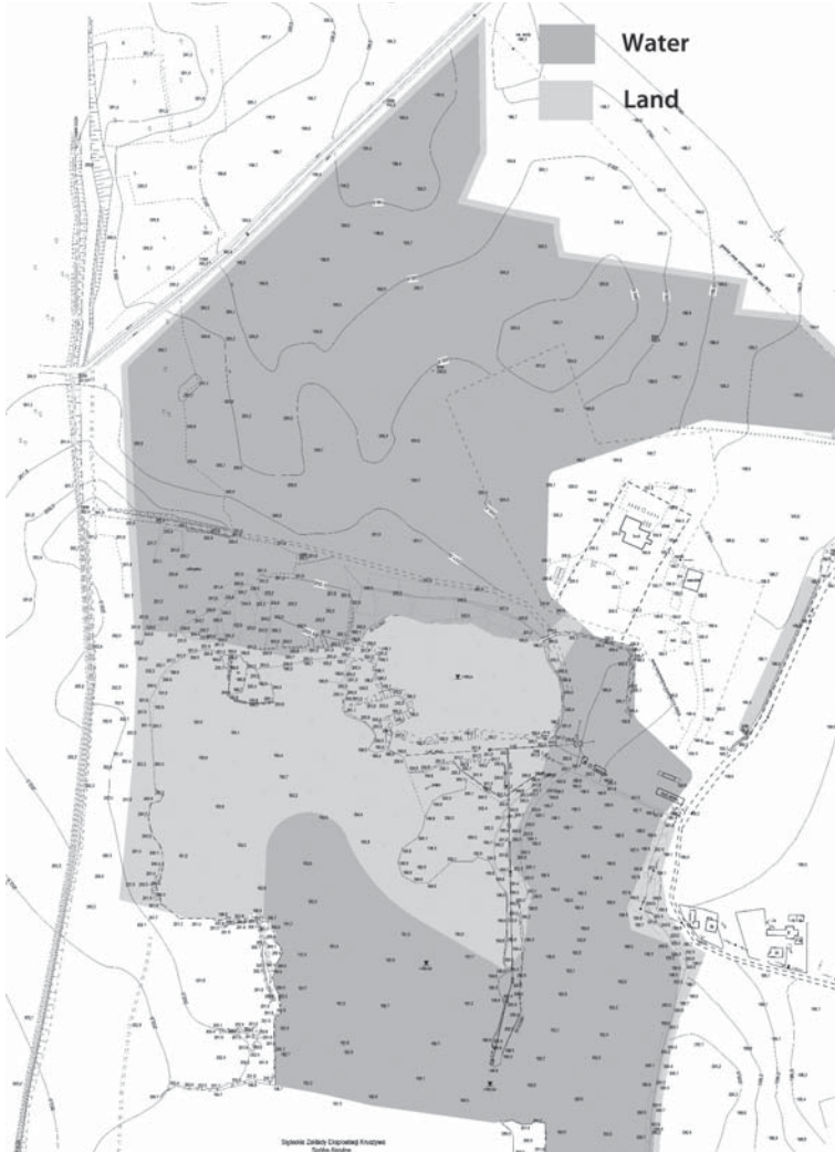
Fig. 4. The map for the project of the “Dębina Łętowska I” deposit development plan providing for a set-up of two reservoirs 8 to 10 metres deep [1]
