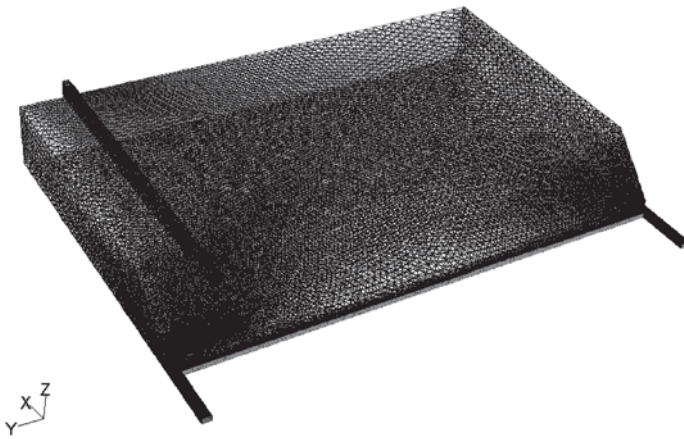
Fig. 2. Meshing of calculated region
