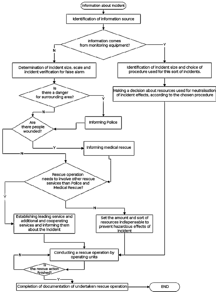
Figure 2. General procedure used in case of incident requiring conducting a rescue operation
