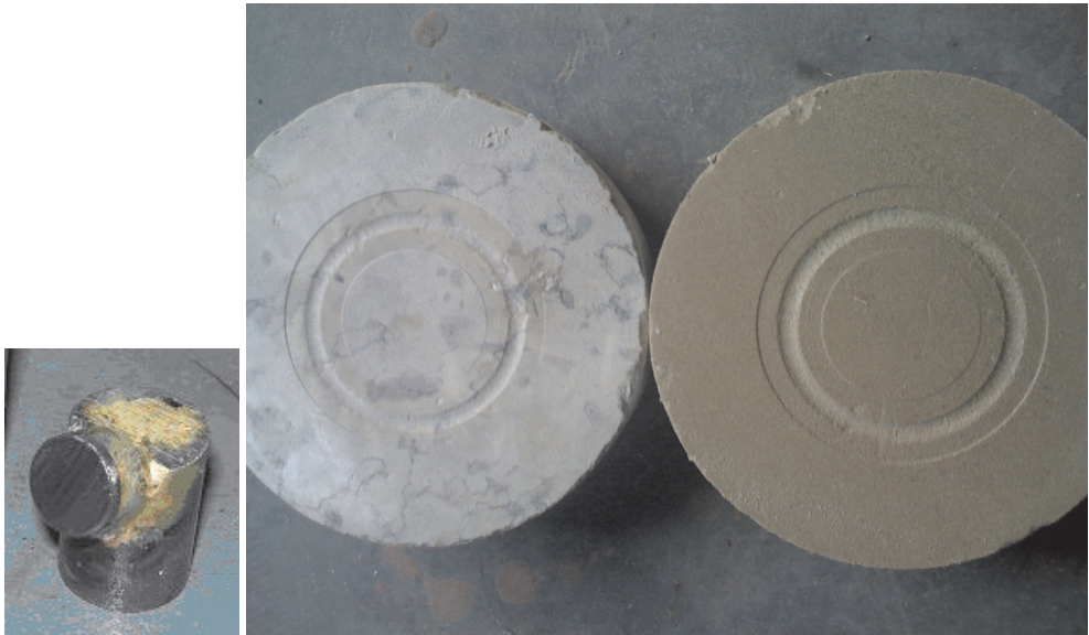
Fig. 3. PDC cutter used in tests (Left). A Carthage Marble (Left) and an Indiana Limestone sample (right)
