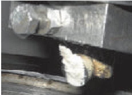
Fig. 6. Cuttings stuck to the cutter (Carthage Marble) (a), Ribbon shaped (Saw Tooth Shaped) cuttings (b)
