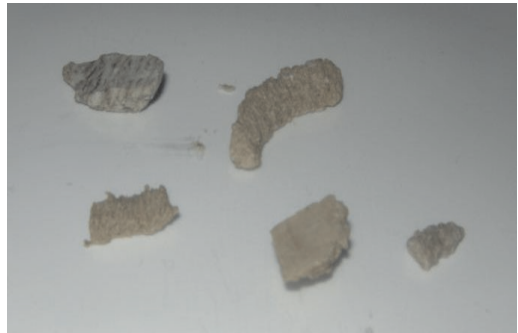
Fig. 6. Cuttings stuck to the cutter (Carthage Marble) (a), Ribbon shaped (Saw Tooth Shaped) cuttings (b)
