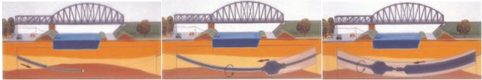
Fig. 1. Horizontal Directional Drilling. Source: Burkacki-Beta-Boring, Warsaw
