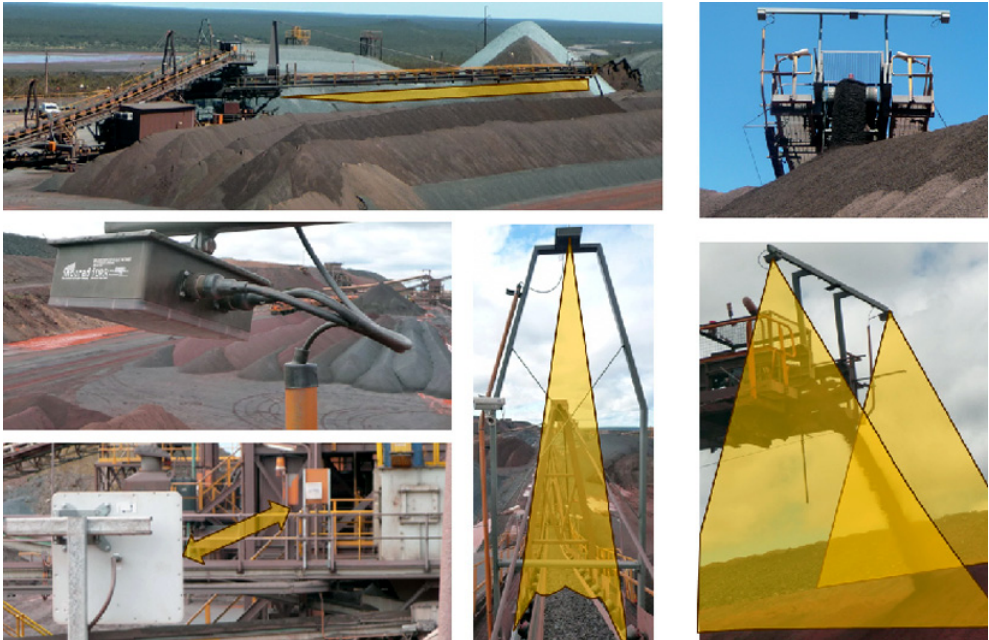
Fig. 11. Tripper with Stacker (top right), Transfer Point Tripper to Stacker for Volume Flow Measurement (top left), Boom with Windrow Cones in background (bottom left), Stacker boom head idler pulley (bottom right)
