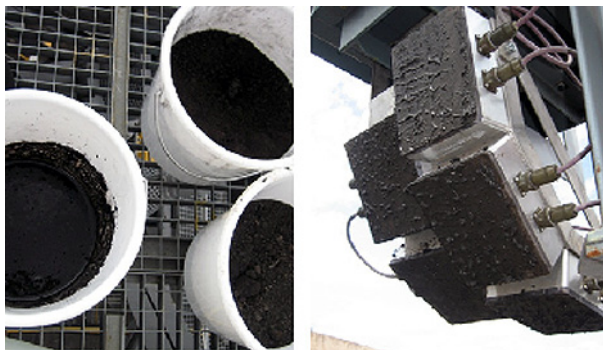
Fig. 3. Radar blockage test with mixture of clay, sand and coal
