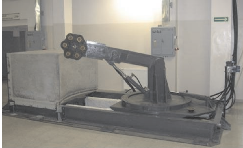
Fig. 4. A view of laboratory stand for testing hard rock mining using single round plate with asymmetrical disc tools (Kotwica et al. 2008, 2009a, b)
