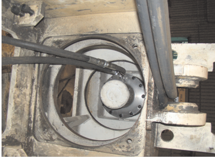
Fig. 16. A view of mounting the hydraulic engine to drive plates with disc tools in the arm of the KR 150 roadheader
