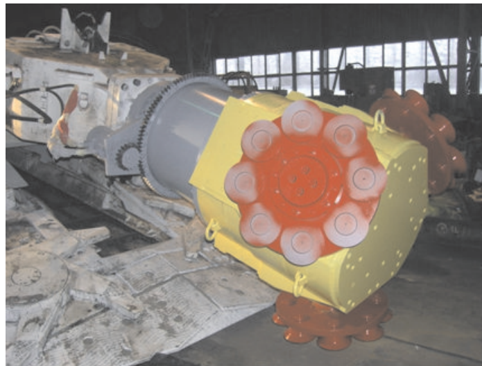
Fig. 11. A view of a head with asymmetrical disc tools of complex motion trajectory on the arm of the KR 150 roadheader, ready for field tests
