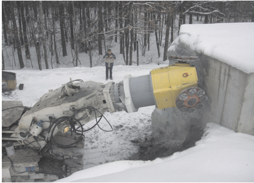
Fig. 12. A view of the KR 150 roadheader with the new solution of a head with asymmetrical disc tools of complex motion trajectory during one of the field tests
