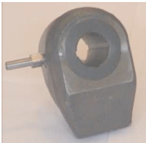
Fig. 8. View of modernized, lubricated holder for the tangential rotary tools of the RM 8 system used for tests (Bęben et al. 2001; Kotwica, 2003, 2005)
