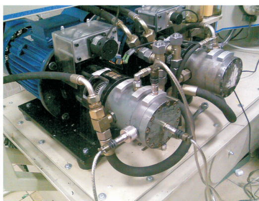
Fig. 7. Distribution of measurement transducers on the tested pump body, and example of acceleration vibration courses for three measurement axes
