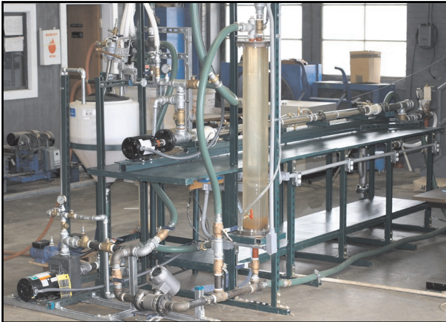
Fig. 2. Small Scale Loop in the Horizontal Position
