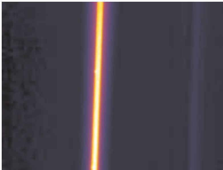
Fig. 2. Thermographic view of tested wire
