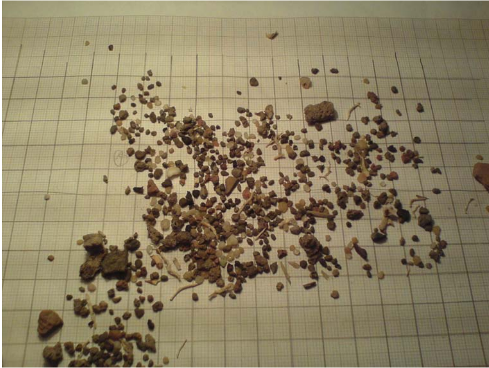
Fot. 1 Examined fraction 0.1-2.0 selected from tested samples
