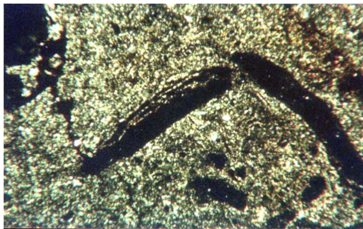
Photo 10 Microscopic picture of tested slag composed of minerals typical for local, thermally changed silt. Polarizing light microscope, Polaroids X, magnification about 80 x.
