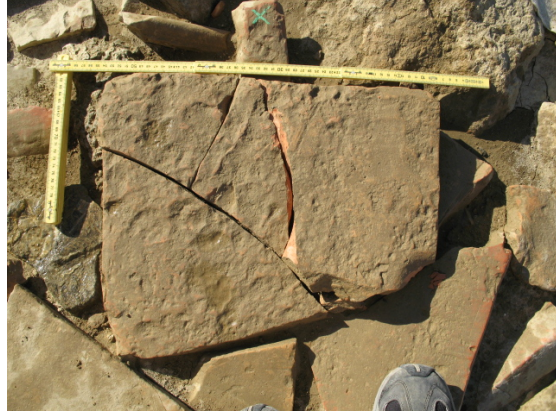
Photo 5B Crushed plate brick
