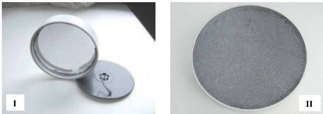
Fig. 4. Example of a sleeve enabling investigating the sound absorption coefficient of granular material: I – sleeve of a diameter 100 mm and thickness 20 mm, II – sleeve filled with granular material (polypropylene)
