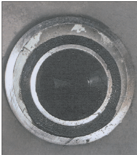
Fig. 5. Swell technology has filled in the un-cemented area [7]
