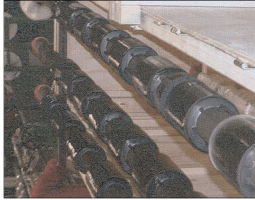
Fig. 3. Expandable zonal isolation profiler tool with feed-through capability for control liners [5]
