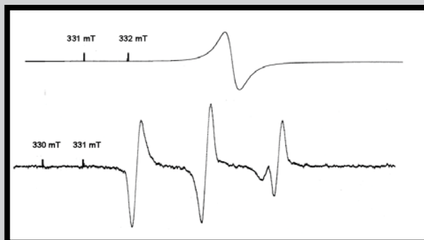
FIG. 4. EPR spectra of coal oximetric probe and TEMPO located in the cells irradiated during 15 minutes by laser at the presence of photolon.
