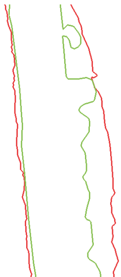
Fig. 1. Change of shape of the river-bed in years 1977–2009, section between cadastral units Czernichów and Pozowice
