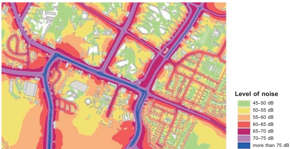
Fig. 1. Section of a noise map for the city of Olsztyn ( L_{DWN} for road traffic)
