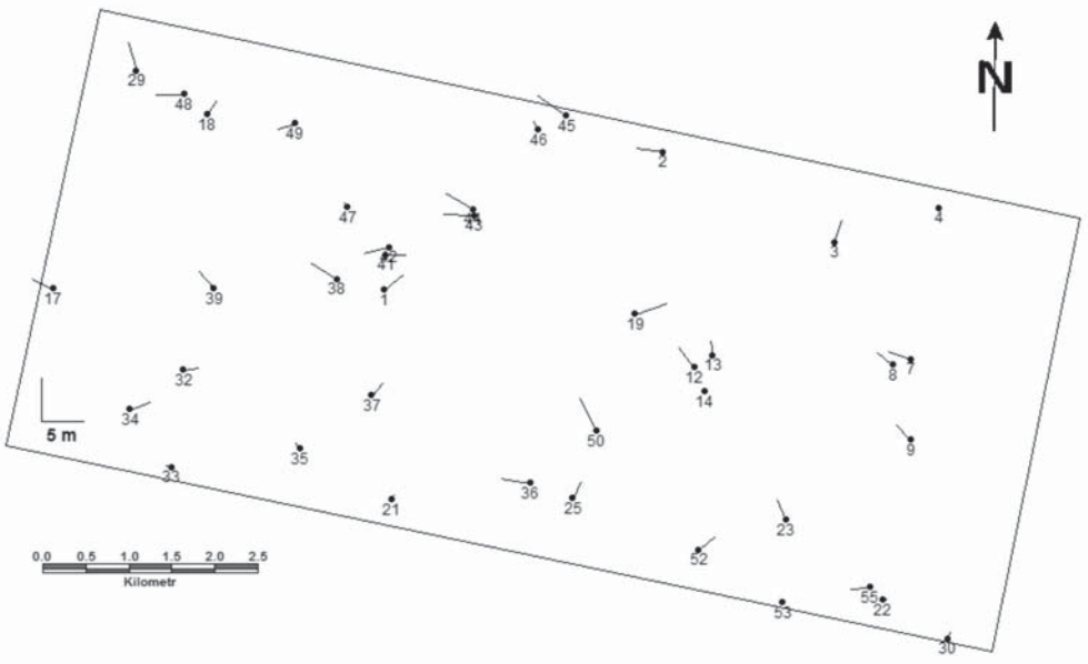
Fig. 3. Check points deviations for TSX-2 orthoimage generated based on one point and DTED-2 model
