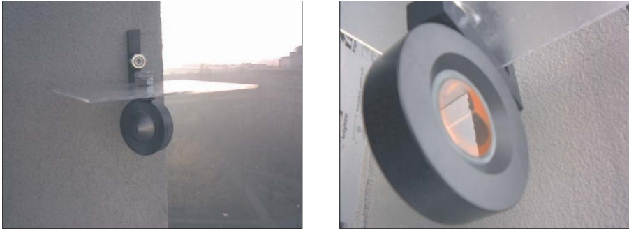
Fig. 2. Exemplary installation of circular prisms
