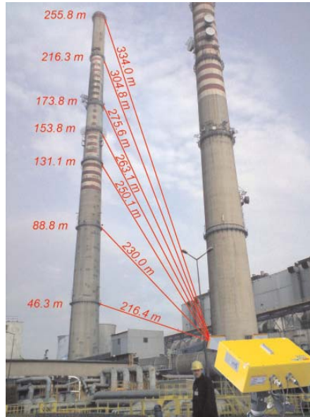
Fig. 3. Microwave interferometric radar during dynamic testing of K2 reinforced concrete chimney of H = 260 m
