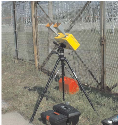
Fig. 1. Microwave interferometric radar during surveying procedure
