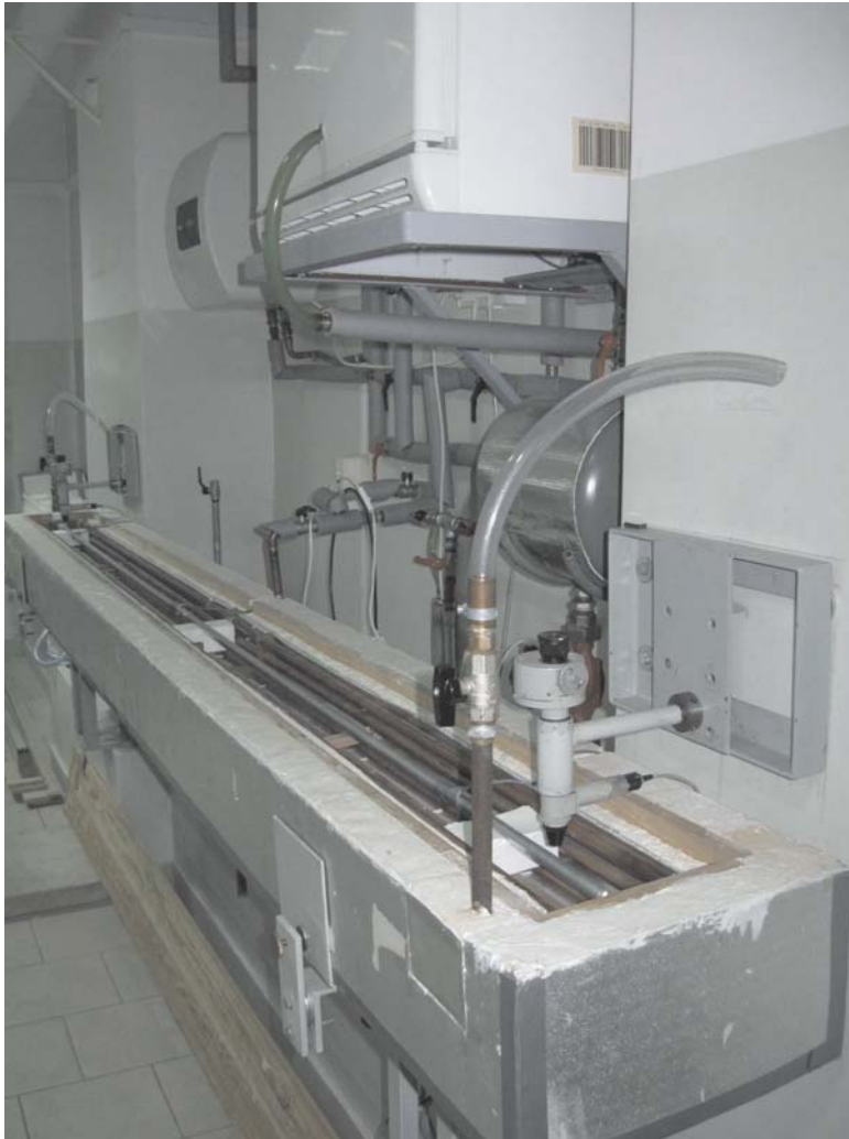
Fig. 2. Stand for determining the coefficient of linear thermal expansion
