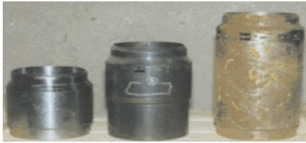
Fig. 12. Core breaker Christensen – spring and combined
