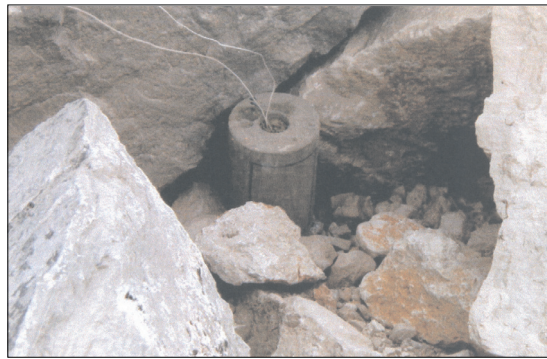
Fig. 7. Laboratory core plug N° 6966 photographed at polygon ready to be blasted by electrically activated a 3 g PCF propellant charge, positioned inside concentric hole
