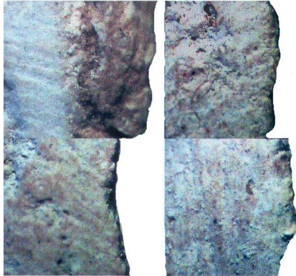
Fig. 5. Various patinated coatings of four examples of limestone blocks from the Hatshepsut Temple. Digital microscope, magnification 5 x.
