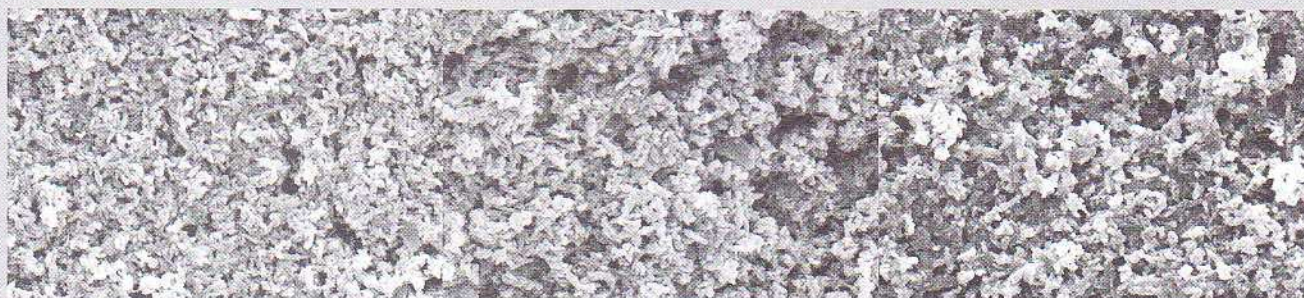
FIG. 1. Nanosize HA crystals in various solvent systems.
