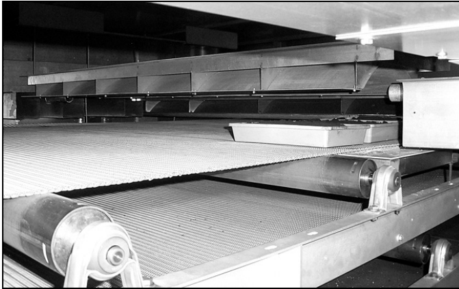
Fig. 2. Setup for microwave radiation coal drying
