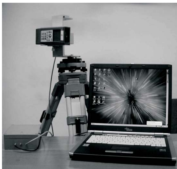
Fig. 8. Laser scanner integrated with a DISTO plus distancemeter set for scanning vertical cross-sections (complete with a recorder - a laptop)
