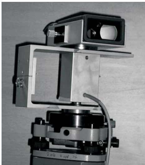
Fig. 7. Laser scanner integrated with a DISTO plus distancemeter set for scanning horizontal cross-sections
